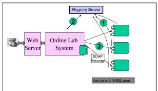
Fig 1. The distributed system framework for online experiments
